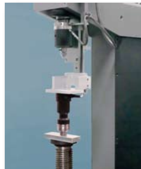
The B.O.S.S. ® Brinell scanner can be integrated with the tester to automatically make an optical Brinell measurement for each test.
