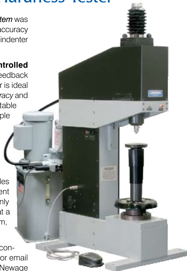
The basic 7000 Series Tester package includes the hydraulic unit and pedal start switch. The system has both an elevating screw and 4" hydraulic cylinder stroke. The elevating screw can be removed to increase the capacity even more.
