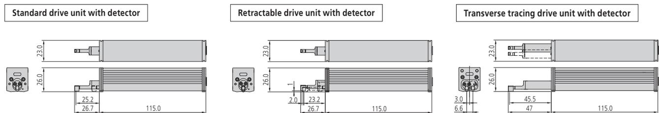
\* External dimensions for the models with standard detector conforming to each drive unit.
