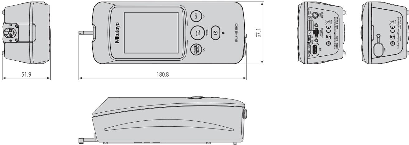
Drive unit not stored inside display unit (Standard detector installed in drive unit)
