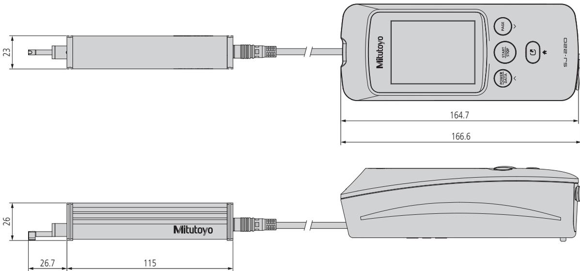
Drive unit attached with detector
