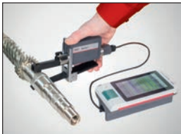
▲ Traverse Drive for Shaft Measurements
