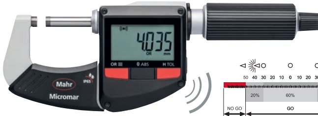
▲ Integrated Tolerance Markers
