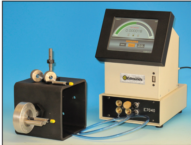
Air “match” gaging for clearance.
