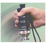
The scope can be turned on and off automatically with the optional motion sensor/timer control, part 5620-05a.
