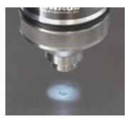
The new LED system directs the light at a shallow angle for optimum, consistent illumination of the impression.
