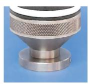
Removable snap-on base can be used for improved stability during testing or removed for use in tight locations.
