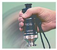
The scope turns on and off automatically with the optional motion sensor/timer control, part 5620-05a.
